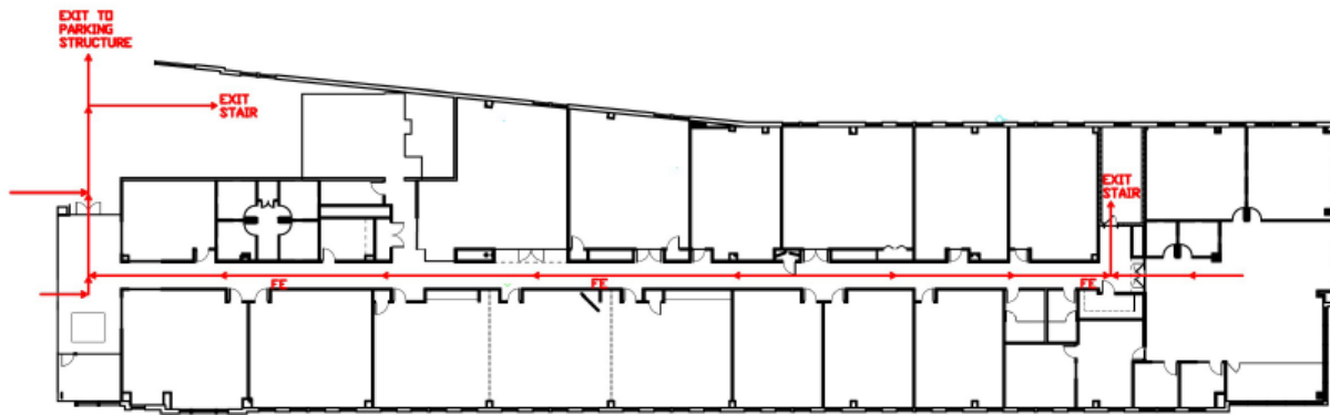
EGRESS PLAN - BAYSHORE EAST FE=Fire Extingulsher
